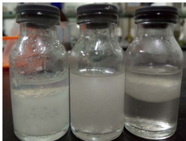
Figure 5. Pictures of DEHP Pickering emulsion stabilized by \text{SiO}_2 nanoparticles after placing for 36 h at \text{pH} \sim 4, 7, 10 (from left to right), respectively. [Color figure can be viewed in the online issue, which is available at wileyonlinelibrary.com .]
